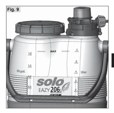
Fill the tank no further than to the upper-most mark (**MAX**) of the spray tank.
