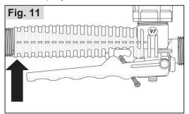
To spray, depress the hand lever on the valve. Release the hand valve lever to stop spraying.
