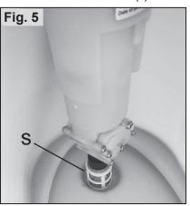
The intake screen (s) is pushed on at the intake manifold to the pump of the spraying agent tank.
