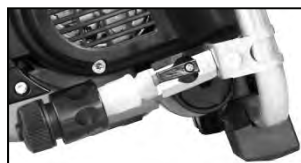
water supply opened (valve lever parallel)
