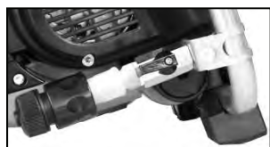
water supply opened (valve lever parallel)
