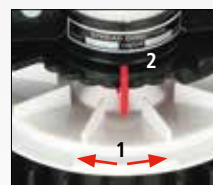
Adjustable throw direction (1), agitator (2)
