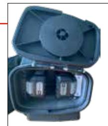
Battery compartment for operating battery and space for a spare battery
