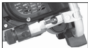
water supply opened (valve lever parallel)
